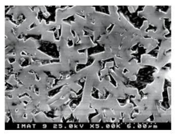
Fig. 6- Typical microstructures of mullite-based recycled samples: (a) sintered at 1250°C; (b) sintered at 1650°C. In this sample the intergranular region was covered by the glassy phase, being mostly removed by chemical etching.
