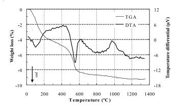
Fig. 2- TGA and DTA curves of the mullite-based recycled composition.
