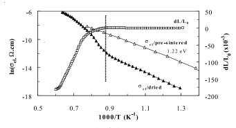
Fig. 4- Dilatometric curve (dL/L<sub>0</sub>) of dried mullite-based recycled sample and Arrhenius-type plot ( $\sigma_{e'}$  estimated by IS) of the same composition dried and pre-sintered at 1350°C.
