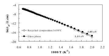
Fig. 5- Arrhenius-type plots of the mullite-based recycled sample, presintered at 1650°C, and of the synthetic glass having the same chemical composition (estimated by EDS) of the intergranular glassy phase present in the recycled bodies.
