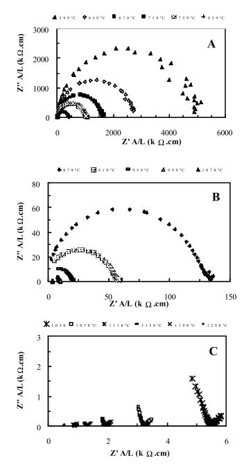
Fig. 3- Impedance spectroscopy evolution with the sintering temperature of extruded and dried mullite-based recycled samples.
