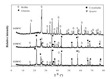
Fig. 7- XRD patterns of powdered samples sintered at three different temperatures for 1 hour.
